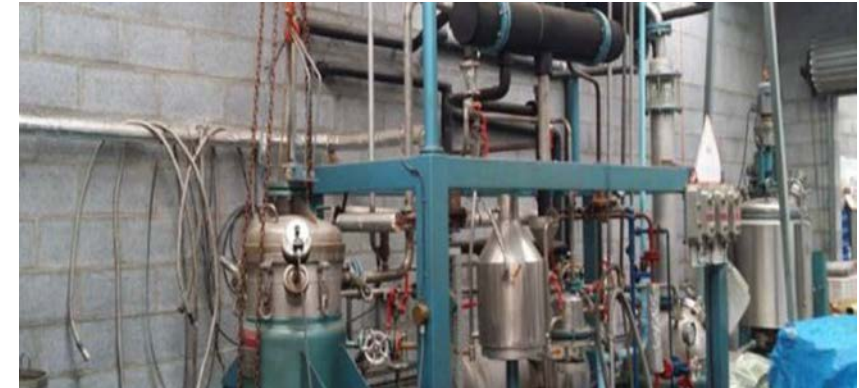
Pilot scale supercritical CO 2 extraction plant at the University of Tasmania is to be used by Martha Jane Medical to develop a proof of concept for a commercial scale cannabis extraction plant
