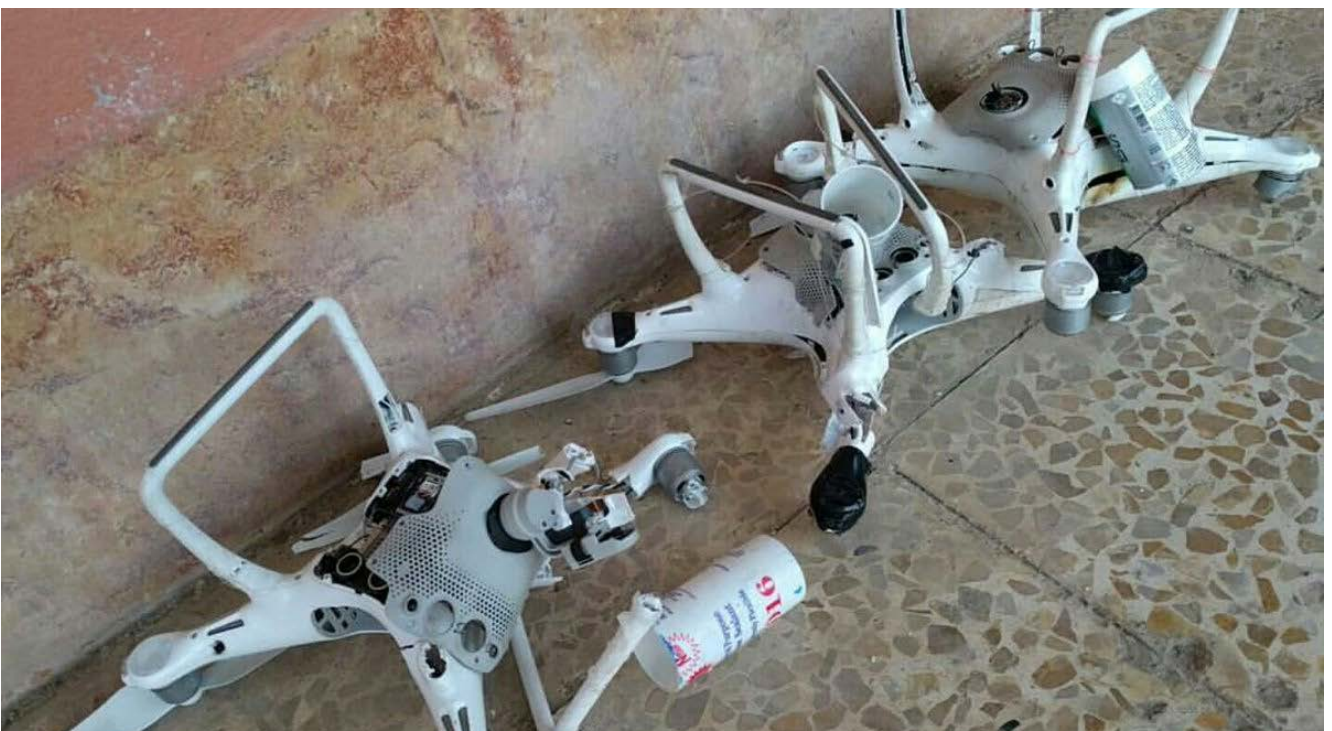
Image: Basic plastic tubes positioned underneath quadcopters appear right size for 40mm grenades
