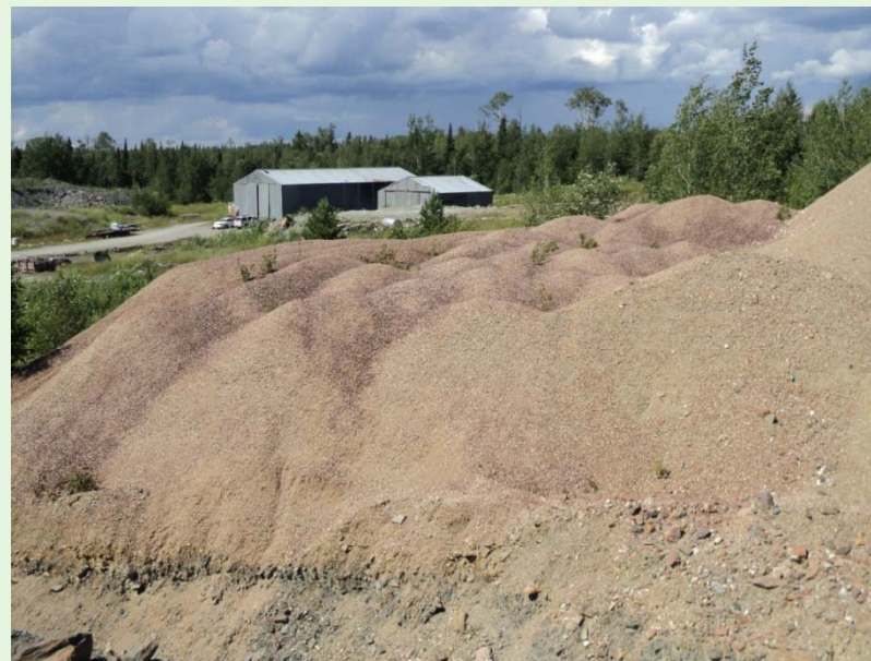
Stock-pile of ore from underground exploration and development at the Cameron Gold Deposit during the 1980s. Stock-pile comprises approximately 21,000 tonnes at 4.2g/t gold for circa 3,000 ounces of gold.
