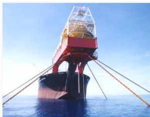
The FPSO, showing the single-point mooring.
