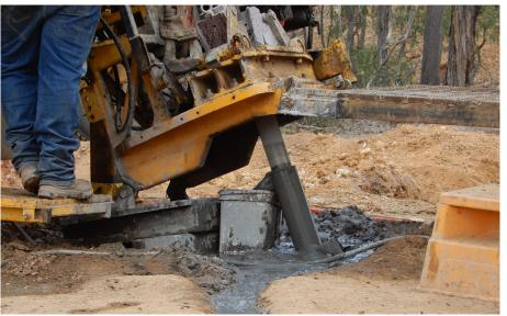
By XRF sampling the water return line on the drill rig we can quickly see indicators which have excellent correlation to lab assay results (lab assay left sludges right on adjacent figure) providing confidence to proceed without waiting for the lab.
