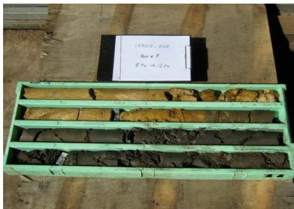
Hangingwall contact with highly weathered gneiss passing directly into completely weathered graphitic schist
