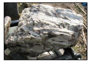
Sample of large high grade spodumene crystals exposed at North Aubry prospect, Seymour Lake, Ontario Canada.
