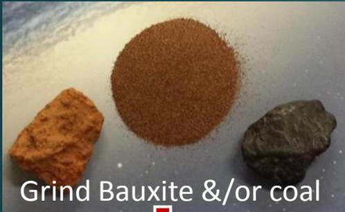
**Bauxite &/or coal ash** =  $36\% \text{Al}_2\text{O}_3 + \text{Fe}_2\text{O}_3 + \text{SiO}_2 + \text{TiO}_2$
