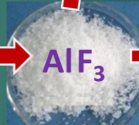
$AlF_3$  electrolyte for Lithium-ion batteries
