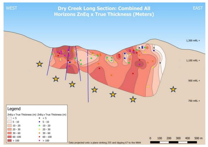
**Figure 1:** Long section showing the true-width grade thickness of the combined massive sulphide lenses that make up the Dry Creek deposit projected onto an inclined plane, highlighting the growth potential for the deposit at depth and the planned drill test pierce points (stars) at a nominal 200m spacing.
