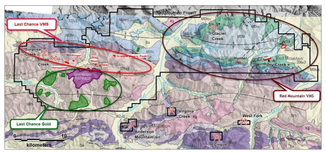
**Figure 2:** White Rock's Red Mountain – Last Chance project showing the four areas of focus for drilling: Dry Creek deposit, the Red Mountain VMS "camp", the Last Chance "VMS "camp" and the Last Chance IRGS gold targets.
