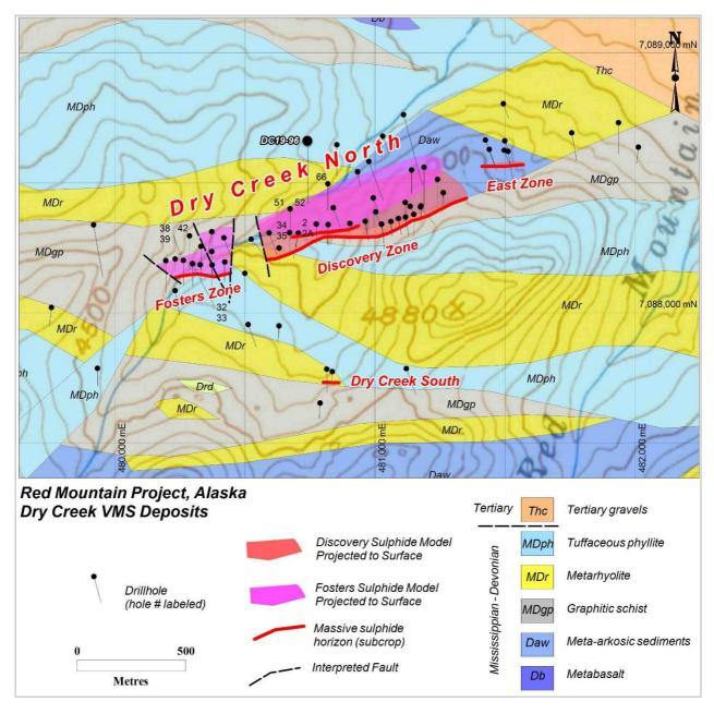
**Figure 2:** Dry Creek prospect showing surface projection of massive sulphide mineralisation lenses and the location of DC19-96 with respect to all historic drill hole traces on the DGGS geology map (after Freeman et al., 2016).
