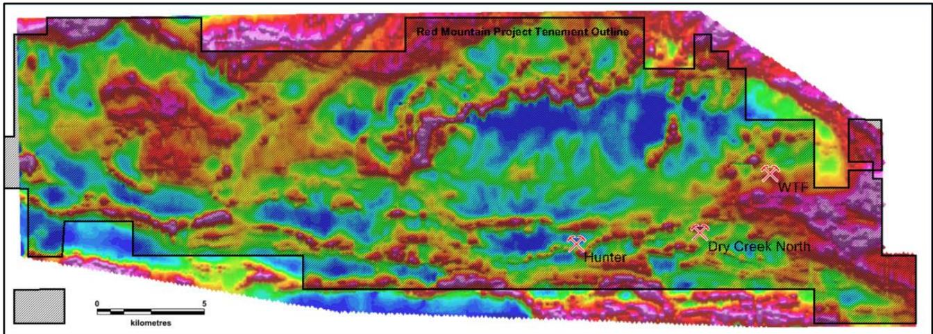
**Figure 1:** Preliminary image of SkyTEM airborne EM survey (channel 30) over an area of 500km<sup>2</sup> centred on the Bonnifield East district with the location for the Dry Creek and West Tundra Flats VMS deposit Mineral Resources<sup>2</sup> and the new discovery at the Hunter Prospect.
