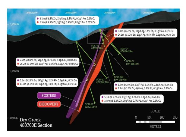
**Figure 3:** Cross-section 480,700E looking towards the east through the Dry Creek deposit showing the geometry of the Fosters and Discovery mineralised massive sulphide lenses and drill intercepts.
