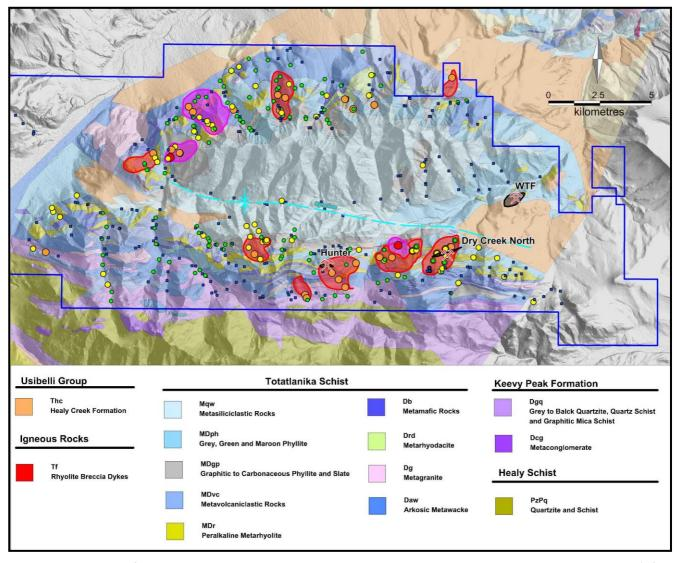
**Figure 6:** Location of high priority stream sediment geochemical anomalies on the DGGS geology map (after Freeman et al., 2016) and terrain surface with locations for the Dry Creek and West Tundra Flats VMS deposits, and the recent Hunter VMS discovery.
