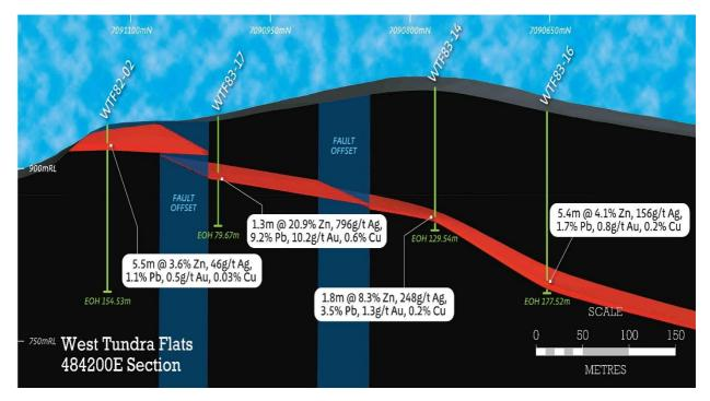
**Figure 4:** Cross-section 484,200E looking towards the east through the West Tundra Flats deposit showing the mineralised massive sulphide lens and drill intercepts.
