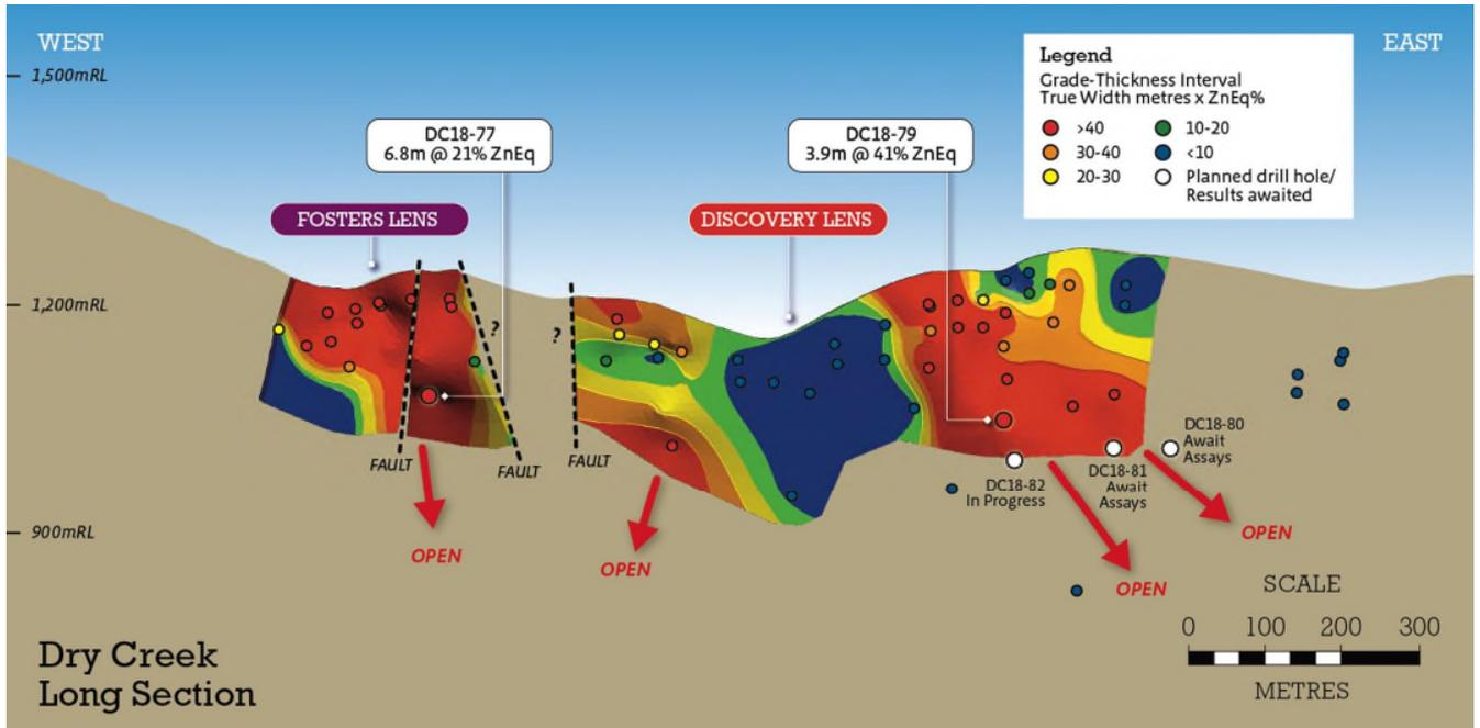
**Figure 2:** Dry Creek long-section looking north showing the Fosters lens (west) and Discovery lens (east) – refer Figure 4 for lens location.
