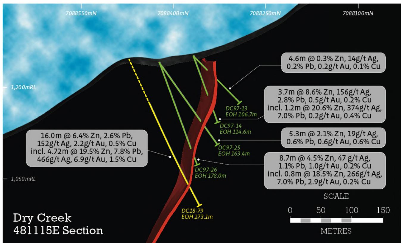
**Figure 3:** Cross-section 481,115E looking towards the east through the Dry Creek deposit showing the geometry of the Discovery mineralised massive sulphide lens and the drill intercepts for DC18-79 (yellow trace) and historic drill holes (green traces).
