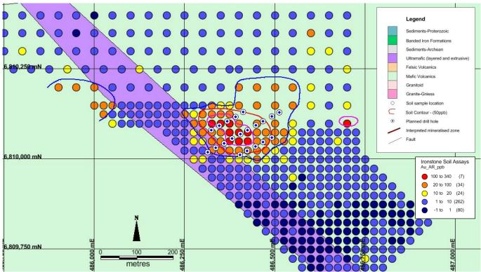
Figure 1: Geology map showing the Ironstone gold soil anomalies and planned air-core drilling locations
