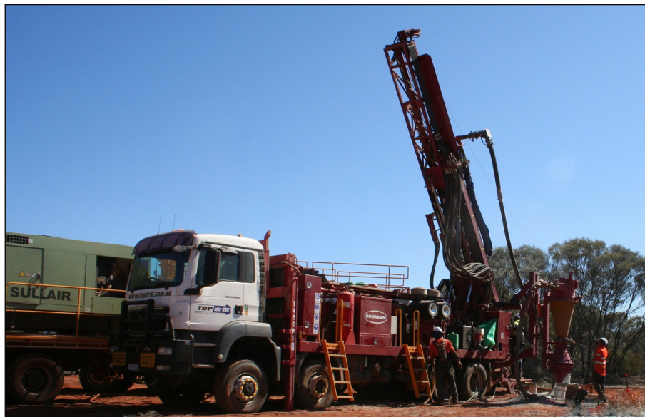
Figure 1 – RC Drilling is being utilised to test key geophysical targets at Curara Well
