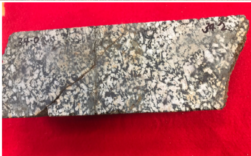
Magnetic grains surrounded by coarse feldspar "getting ready to go rotten"
