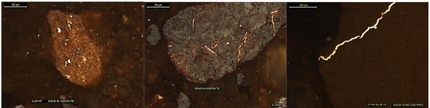
Figure 6: Polished sections of coarse free gold, gold in quartz, gold in goethite, gold in goethite, gold veins in goethite
