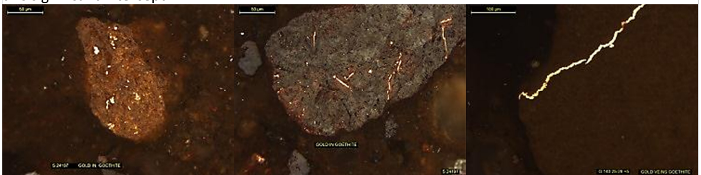
Polished sections of coarse free gold, gold in quartz, gold in goethite, gold in goethite, gold veins in goethite
