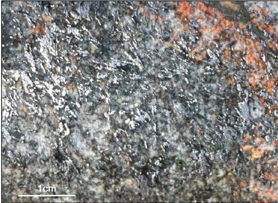
Figure 4: Drill core sample from T12 showing large flake graphite (IVD006, 49m)
