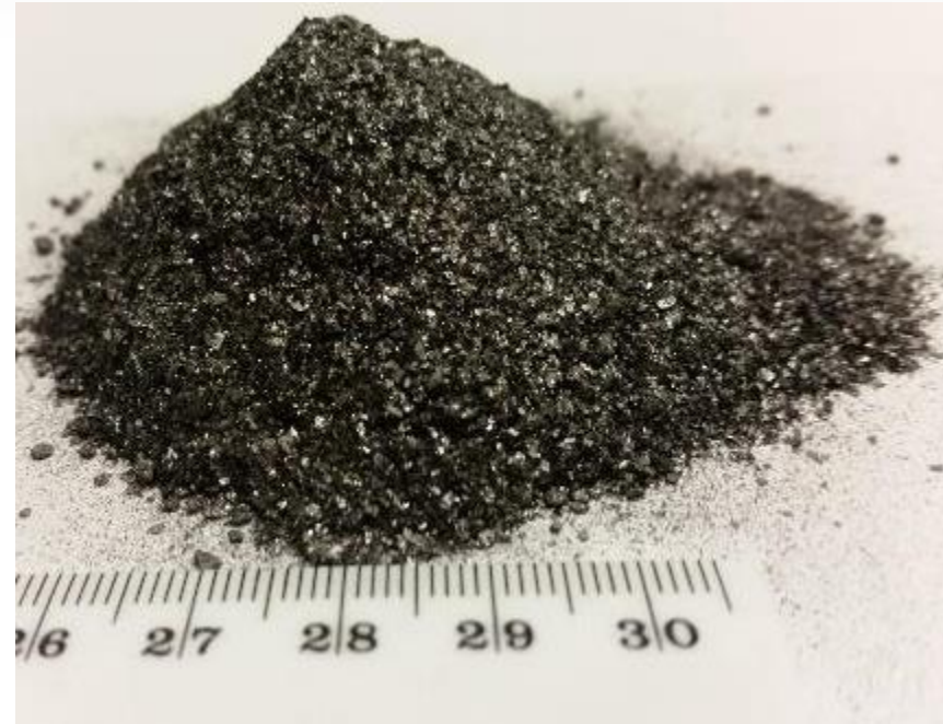
Sample of graphite concentrate from Ancuabe through flotation achieves 98% TGC.
