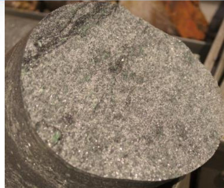
Diamond drill core from Nicanda Hill prospect on License 5966 showing graphite and vanadium
