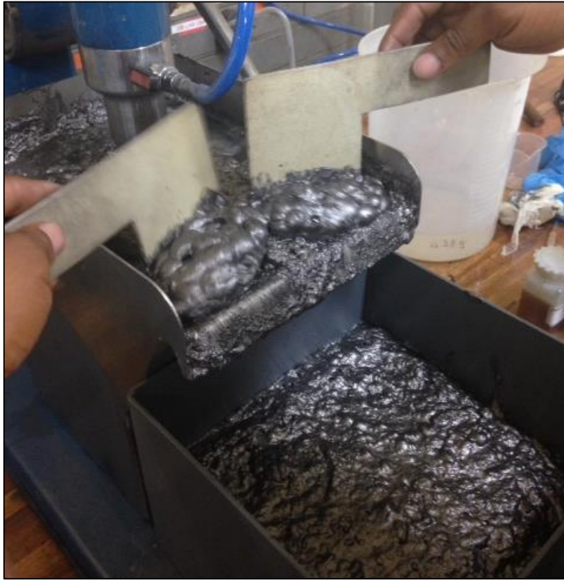
Figure 2. Flotation chamber at Mintek showing the manual recovering the graphite flake concentrate
