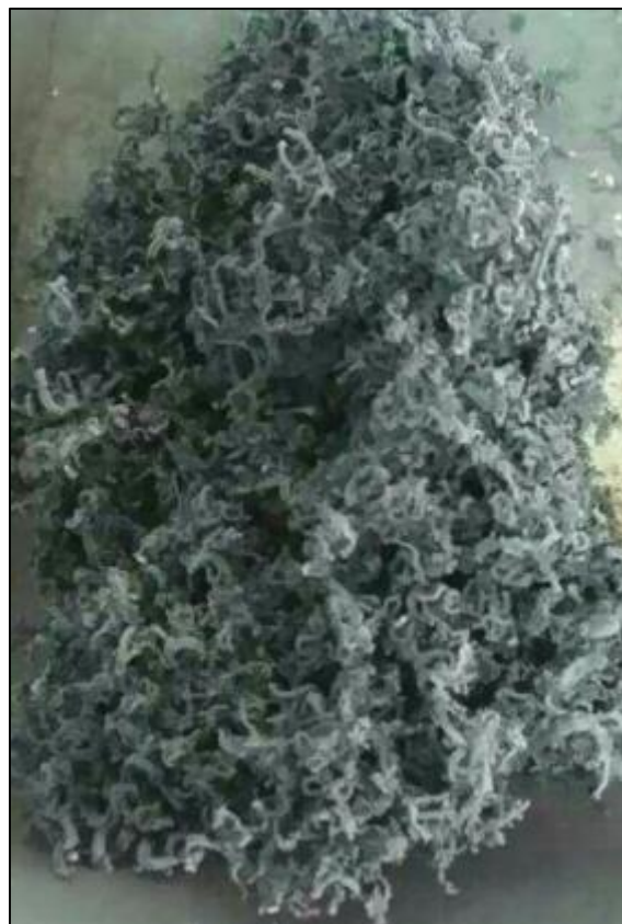
Figure 1. Image of the TMG in expanded form (width of photo is 20cm)
