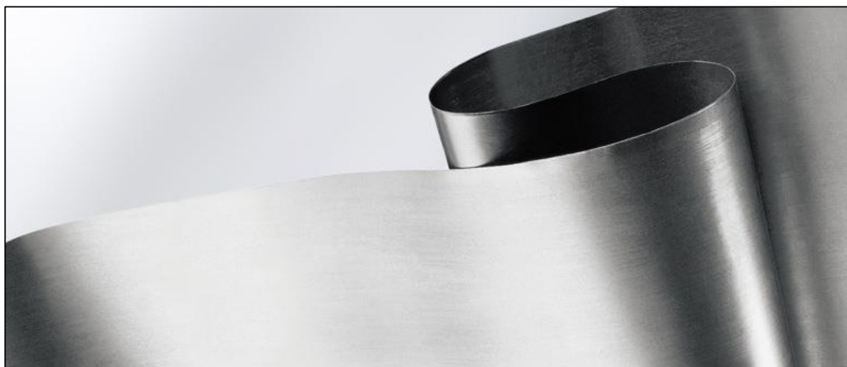
Figure 2. Image of Graphite Foil made from expanded graphite (Sourced. SGL Group, http://www.sglgroup.com )
