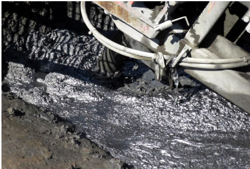
Image of the graphitic material being liberated using a flotation method at the ALS Metallurgy laboratory
