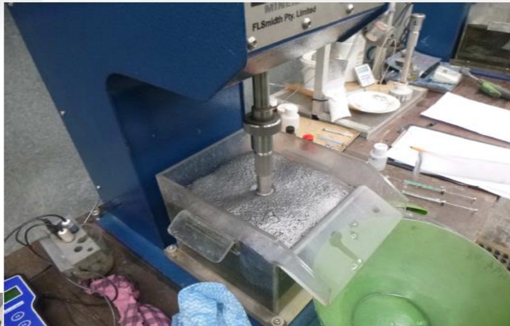
Image of the graphitic material being liberated using a flotation method at the ALS Metallurgy laboratory
