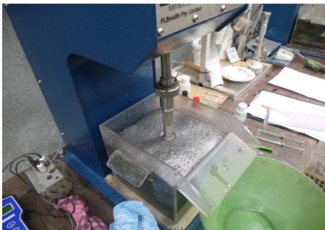
Figure 6. Image of the graphitic material being liberated using a flotation method at the ALS Metallurgy laboratory.
