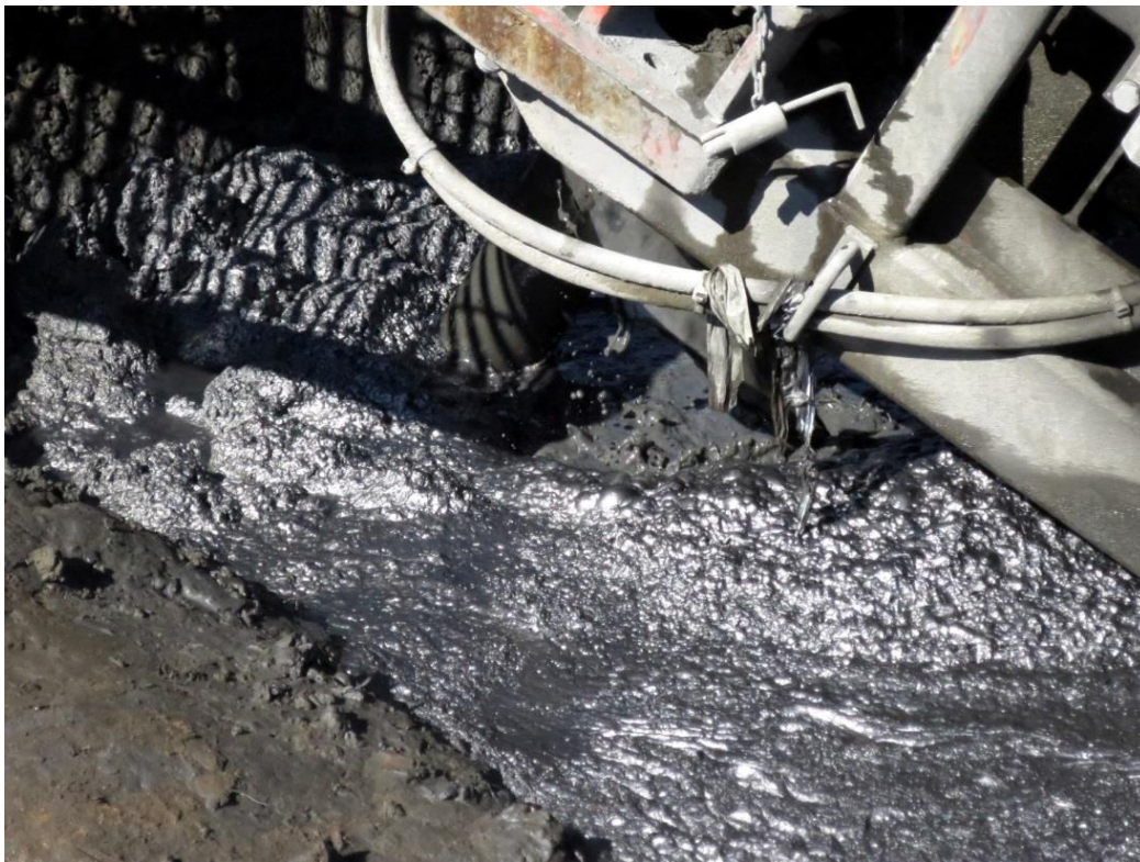
Figure 7. Graphite liberation on as seen at surface on diamond drill hole GBND0005
