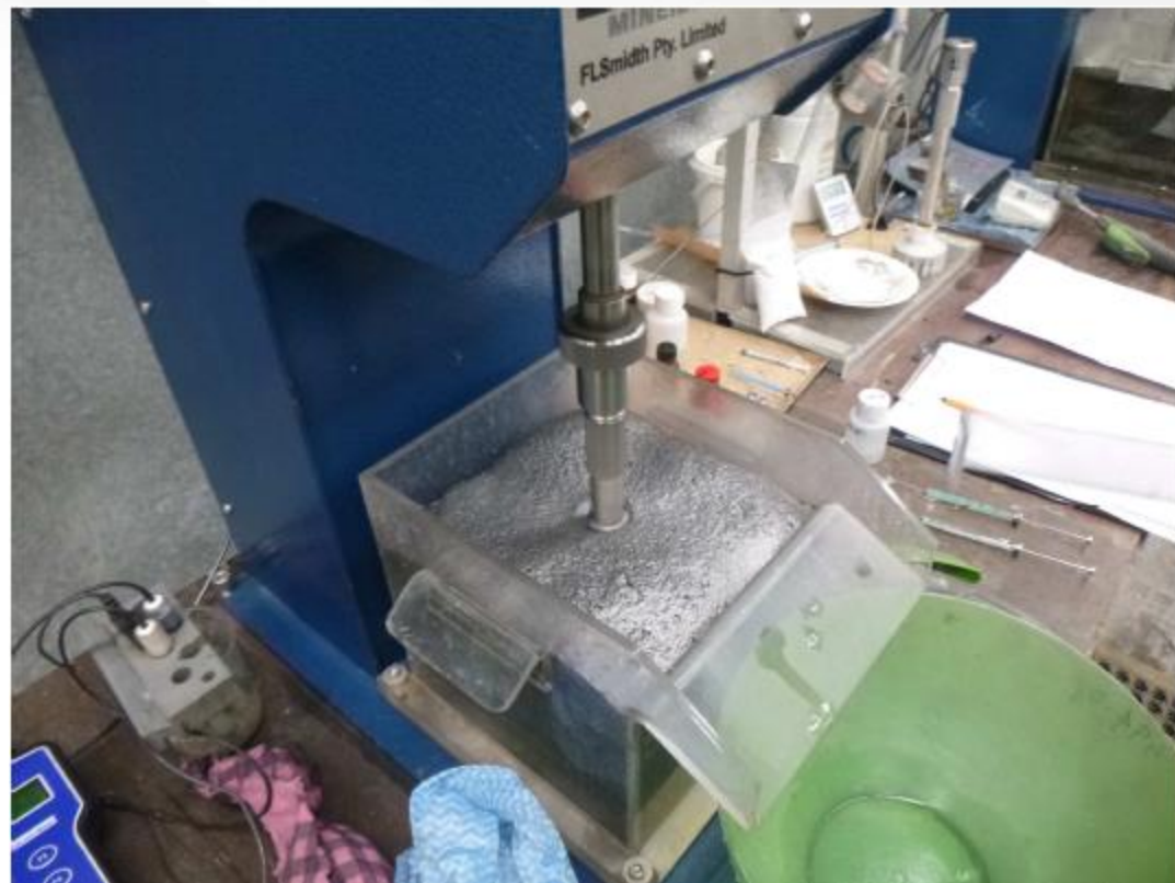
Image 14. Image of the graphitic material being liberated using a flotation method at the ALS Metallurgy laboratory.
