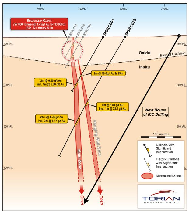
**Figure 5.** Mt Stirling Section 1640 N showing Main Zone, Hanging Wall Zone, and future drill hole trace of future deeper R/C drilling.
