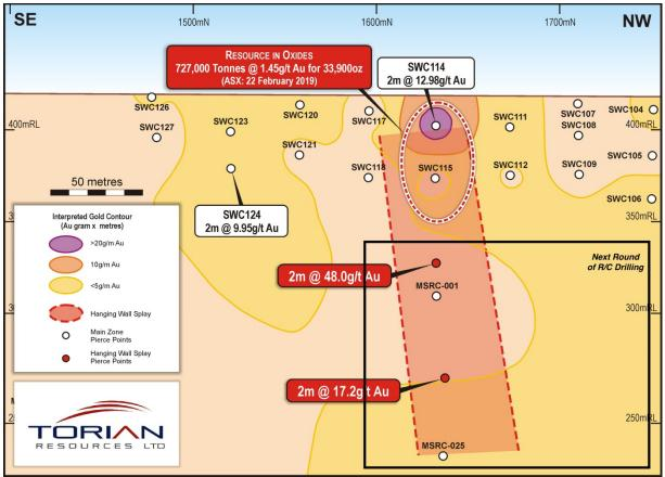
**Figure 4.** Mt Stirling Longitudinal Section showing Grade x Width Contours, Plunge of the Main Zone and Hanging Wall (Red) Zone
