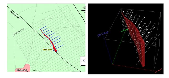
Figure 7: Drilling plan view of Mt Stirling drilling campaign and 3D mineralisation model
