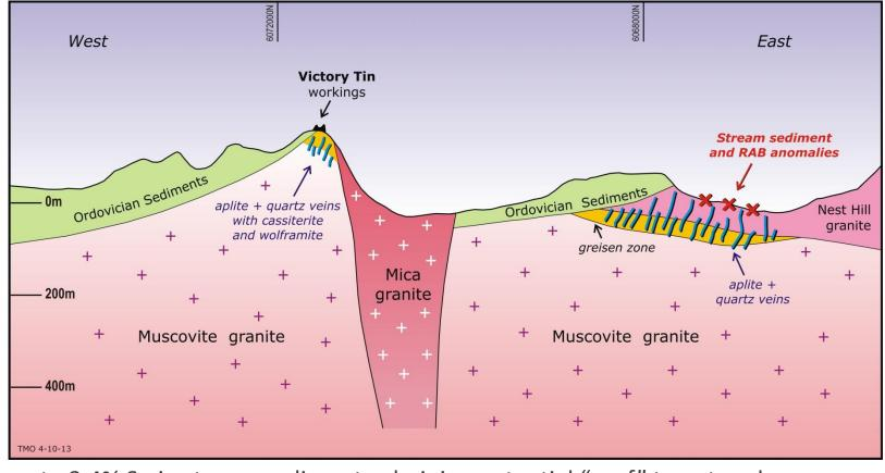
up to 3.4% Sn in stream sediments, draining potential "roof" target under Ordovician sediments
