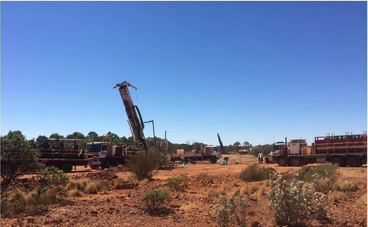
*Figure 1. RC (foreground) and diamond (background) drill rigs at Crown Prince.*
