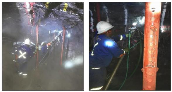
Figures 1 & 2 Show Drilling and Blasting Preparation at Frankfort Mine
