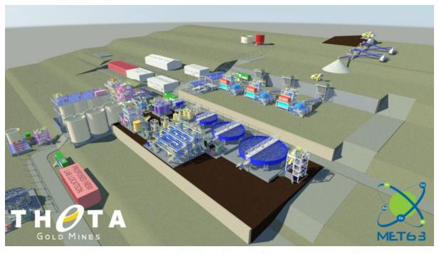
Figure 1: New TGME Plant Layout (ROM/Crush/Grind/Floatation/Oxidisation/CIL/Goldroom/Labs/Offices)
