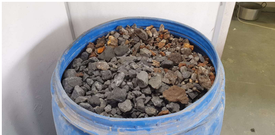
Primary crush product 12mm + via Jaw crusher
