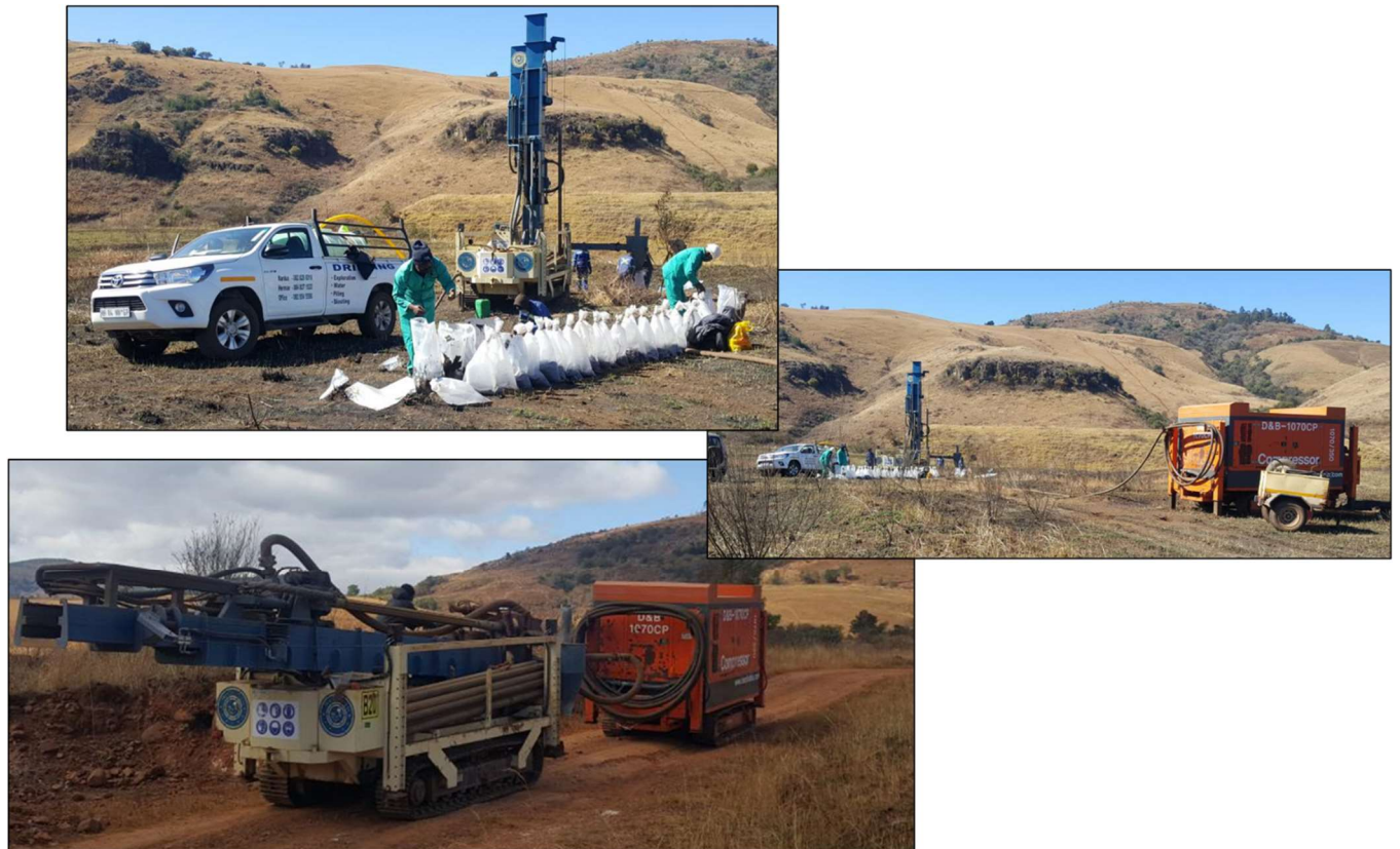
Figure 4: Track Mounted Reverse Circulation Drill Rig and Compressor
