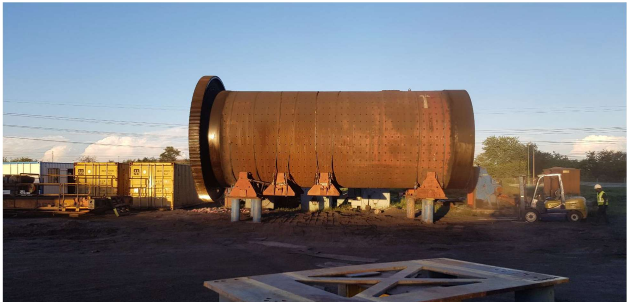
Figure 5: Mill and Containers of Associated Equipment Ready for Transport
