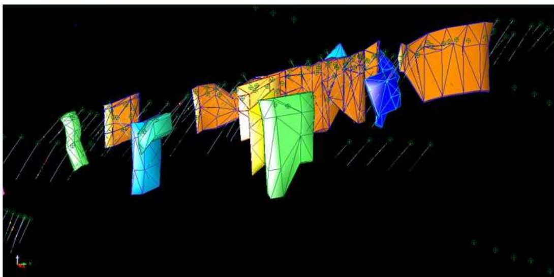
Figure 2 – Taruga Gold Limited - Borobon prospect wireframe interpretation of gold mineralization for preliminary resource estimate.
