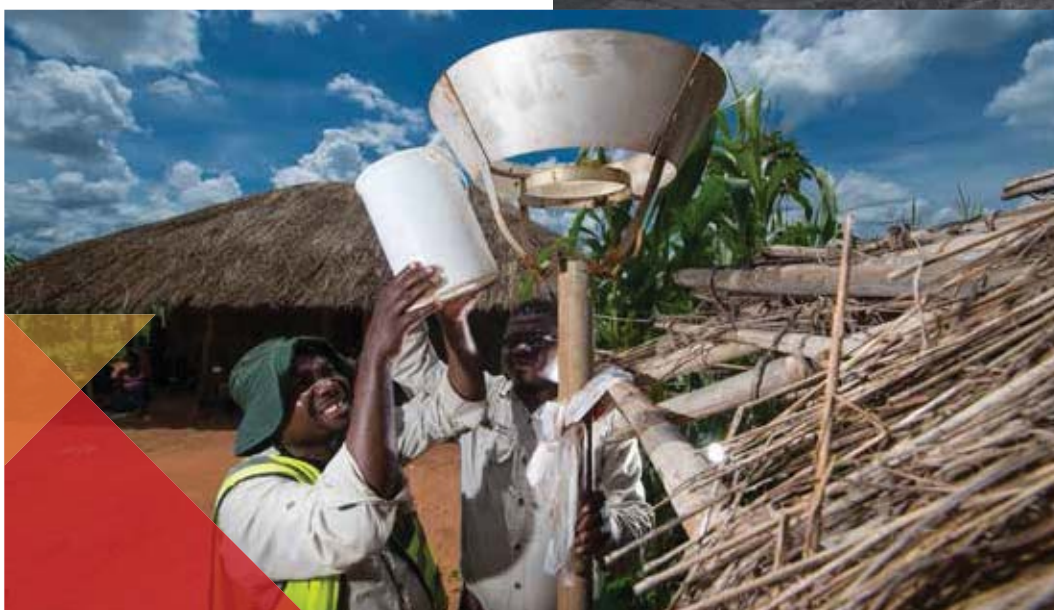
Figure 10: Installation of dust bucket at Balama
