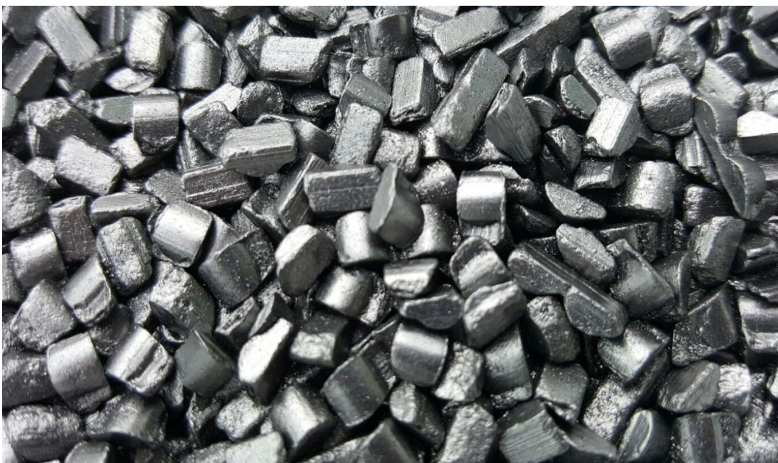
Figure 8: High quality, low impurity Balama natural graphite recarburiser
