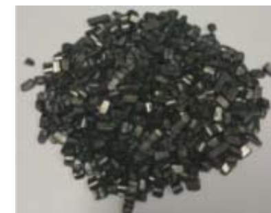
Trial Balama graphite recarburiser briquettes
