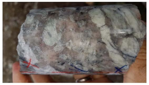
Figure 1: Spodumene mineralisation in the new pegmatite
