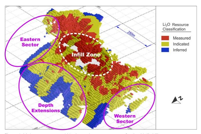
Figure 1: Main target zones within the main resource areas for the 2017 drilling program
