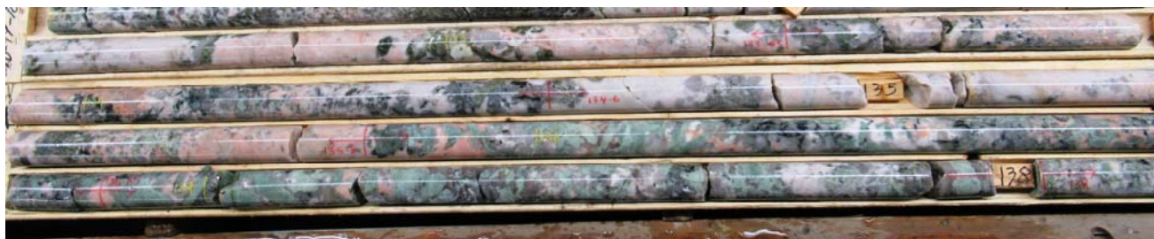
Figure 9: Coarse grain spodumene crystals at deep dyke VD19-10.
