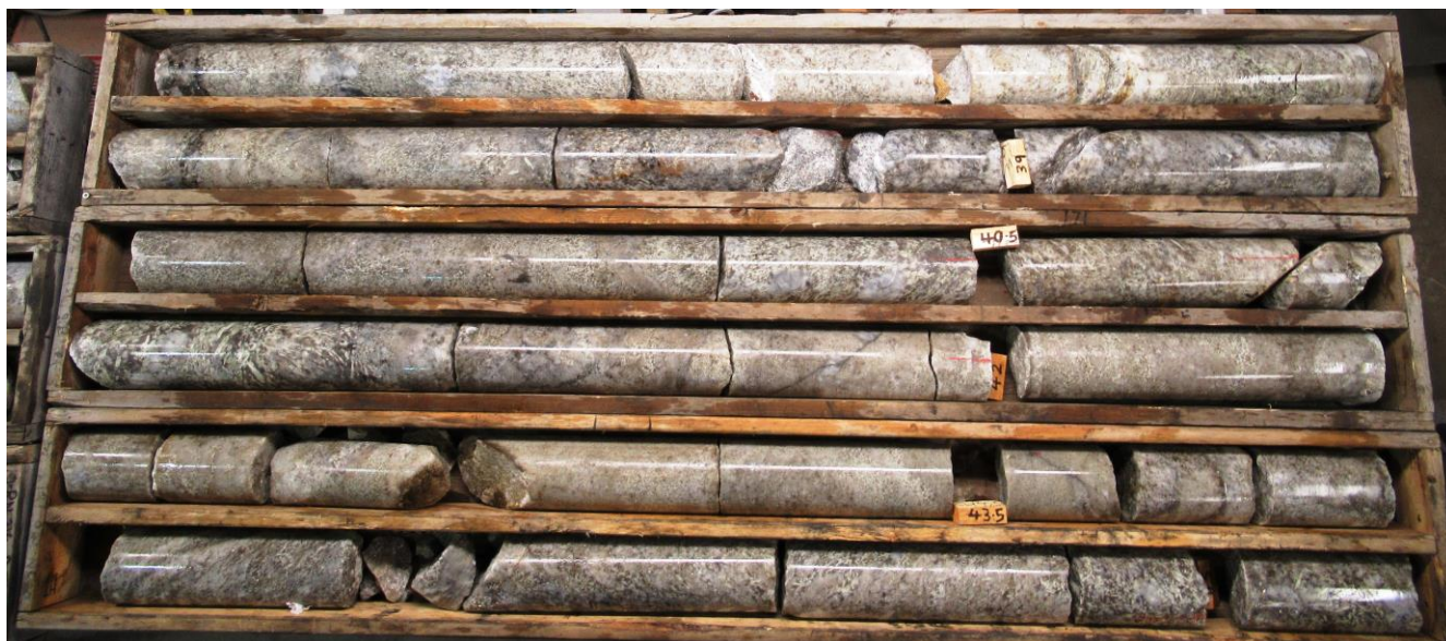
Figure 1: PQ sized diamond core from the first hole in the Phase 3 program Hole 17-32, a twin hole of 16-01 from the Phase 1 drilling program
