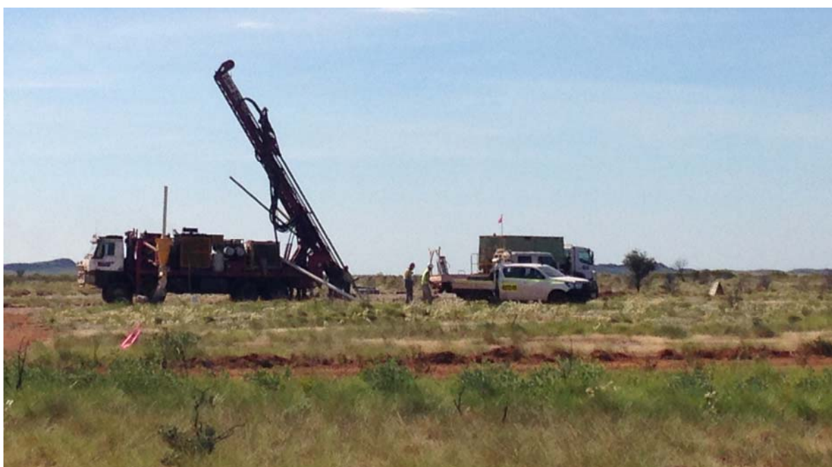
Figure 4 – RC drilling rig on site
