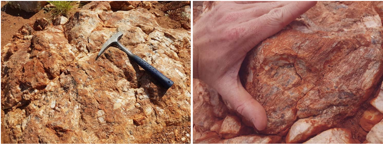
Figure 4: Spodumene mineralisation in the new Eastern Pegmatite
