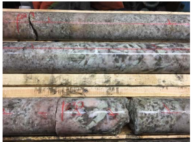
Figure 4: Diamond drill rig on site (left) and diamond core AL-17-005 showing coarse grain spodumene crystals at 229 to 232 metres depth (right)
