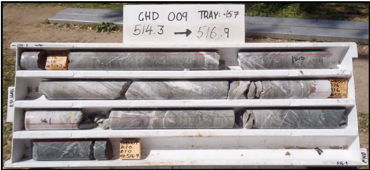
Figure 1: Some of the high-grade gold zone associated with the quartz vein at 516m.
