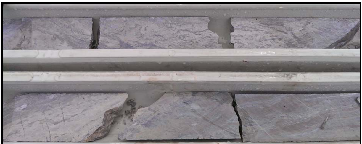
Figure 3: Example of skarnified and altered metasediment at ~548-550m in GHD007. This zone yielded 2m @ 2.67g/t Au.
