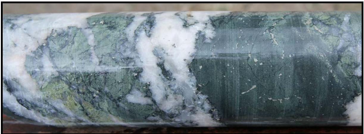
Figure 2: Example of highly altered (chloritised sericite-silica-sulphide) metasediment from ~1,280m in GHD009, showing significant disseminated pyrite and quartz veining.
