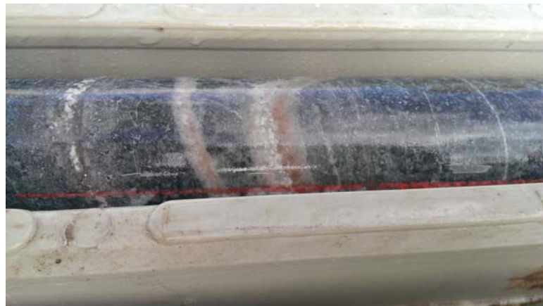
Left: Sericite altered monzodiorite near end of GHD005 and K-feldspar-quartz-carbonate vein at top right of photo
