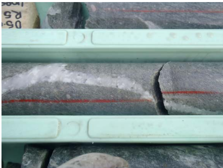
Example of narrow mineralisation style in the mafic diorite unit, below 950m. 15mm wide sulphide-bearing quartz vein with sericite alteration selvage with disseminated sulphide.
