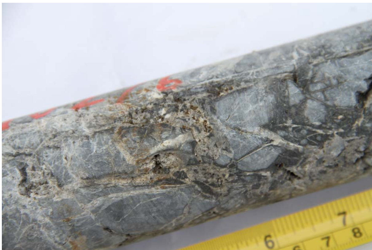
ZK0001 – Quartz sulphide flooded brecciated metasediments from 90.50–90.73 meters (NQ Core 47.6 mm diameter).
