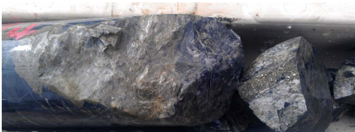
Core of ZK0003–Black Metasediments with sulphide-bearing fingers of grey felsic dykes from 106-107 metres (NQ Core 47.6 mm diameter).
