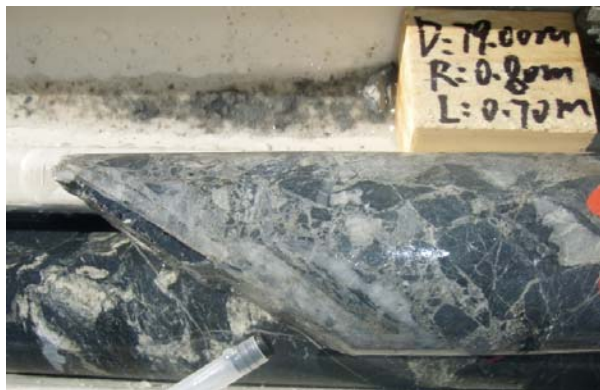
Core of ZK0001–Brecciated metasediments flooded with sulphide-bearing felsic intrusive and quartz veining from 78-79 metres (NQ Core 47.6 mm diameter).
