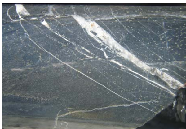
Core of ZK0001–Metasediments with disseminated sulphides and sheeted quartz-sulphide veins from 79-80 metres (NQ Core 47.6 mm diameter).
