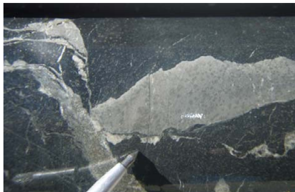
Core of ZK0001–Metasediments with disseminated sulphides and fingers of sulphide-bearing felsic intrusive from 79-80 metres (NQ Core 47.6 mm diameter).
