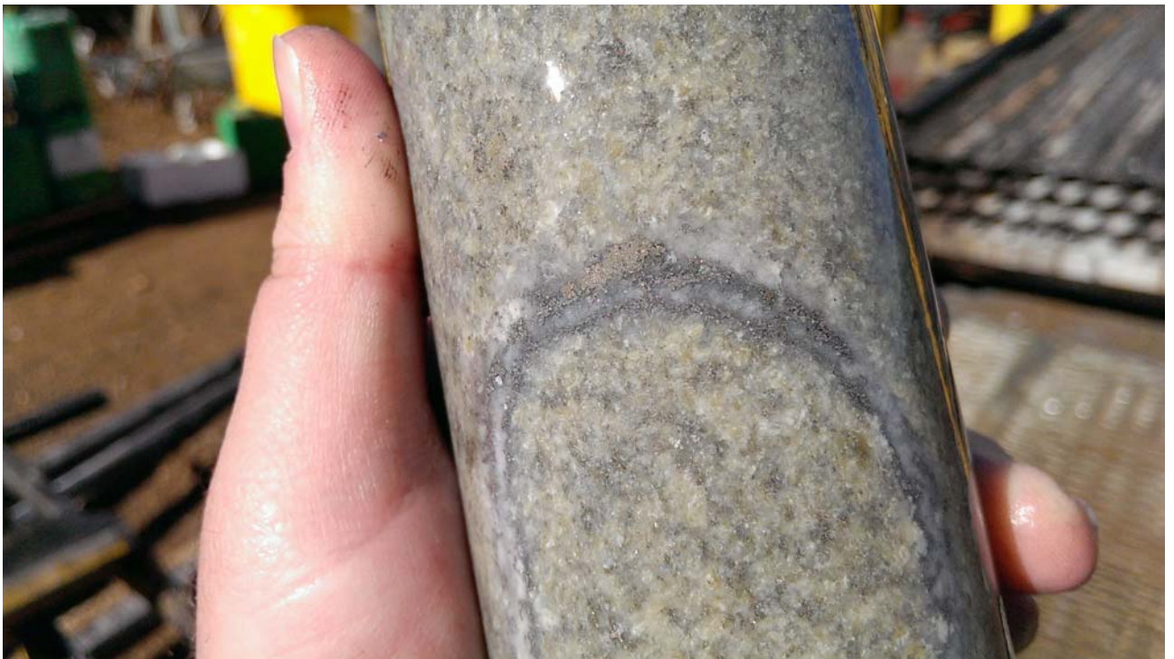
Strongly sericite altered monzodiorite, similar to higher grade core observed from hole GHD001, from approximately 630m with intense arsenopyrite-pyrite mineralisation also associated with quartz veining
