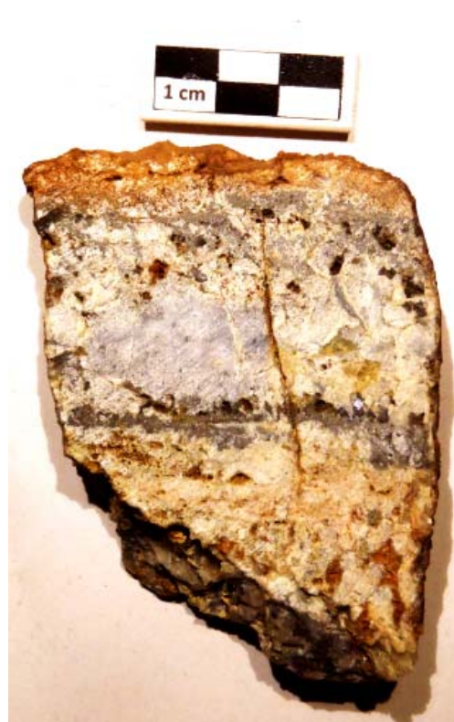
Figure 3: Fraser's Find. Sample S581 (Table 1), High grade quartz-sulphide (abundant arsenopyrite, pyrite, galena) from the dump by the main shaft, assayed 75.2 g/t gold (2.42 ounces), 1,790 g/t silver (57.56 ounces, 1.76 kilograms) and 5.95% lead/tonne (ALS Certificate of Analysis BR12004879).
